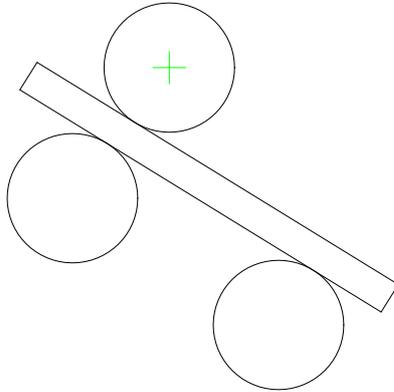
(1), The right roller is in the lower limit position, the left roller moves to the contact workpiece, and clamps the workpiece with the main roller.
