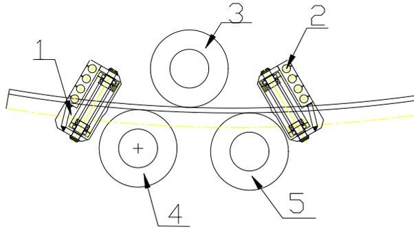
No.: 1, large guide roller    2, small guide roller    3, main roller
