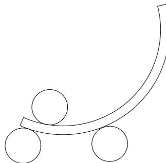
(3), The left roller is down, while the right roller is up, send the material to the left side, and three rollers began to roll, pre-bend between the main roll and the right roller.
