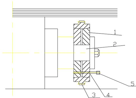
No.: 1, Upper roller shaft    2, Friction block    3, Sprocket
